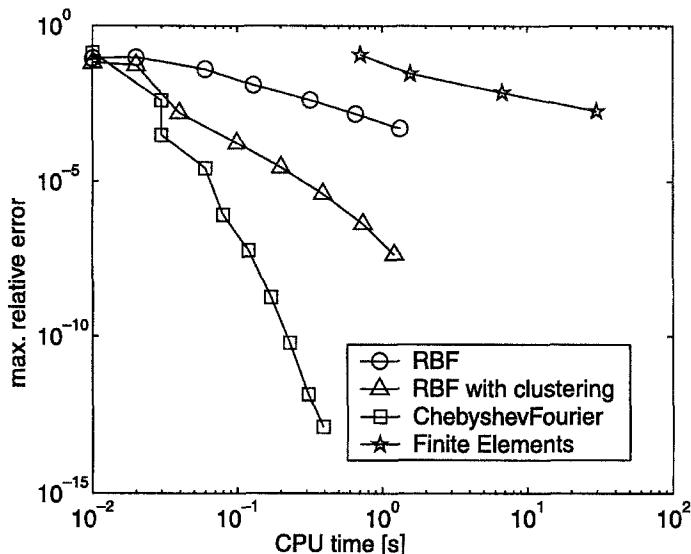
Figure 6. Maximum relative error over the first 12 eigenvalues versus CPU time for the disk with Dirichlet boundary condition.
